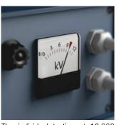
The individual testing at 10,000 volts, in accordance with IEC 60900, ensures safe working with loads up to 1,000 volts.
